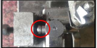
IDEA :-1)Implement the pokayoke for the Job wrong loading At 1st drilling stage 2)job resting pin implement in two step Dia 1st step enter in threading hole & 2nd step Dia resting at job face
